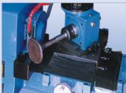
Work head fitted with precision Collet
